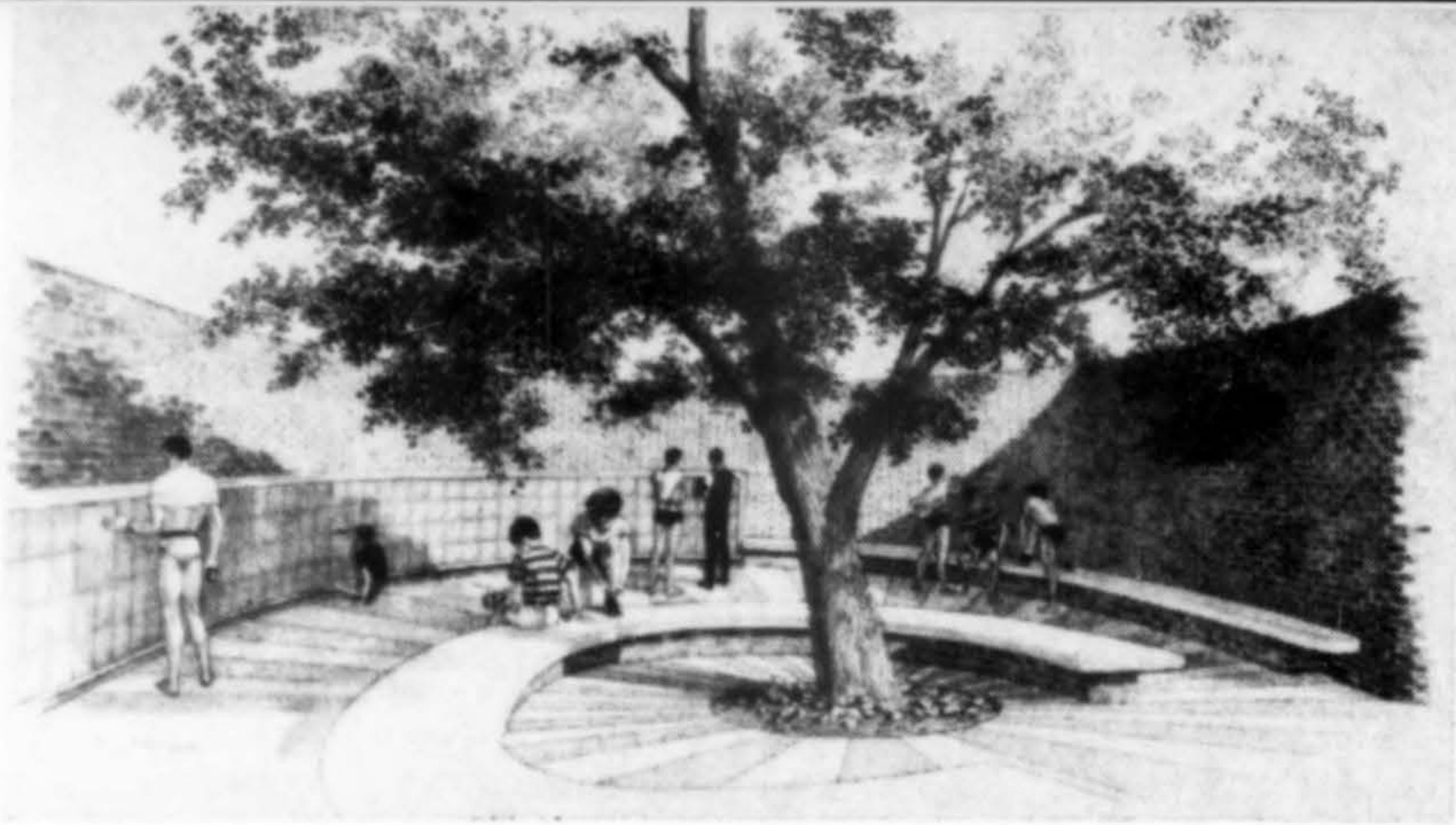
The bath house is predicated on the warm sunny climate. A 10-ft. high curved wall enclosure has no roof.
