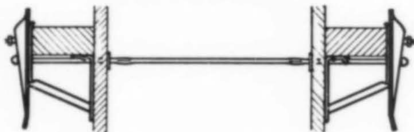
Cross section view shows the simplicity of this system. Note the absence of vertical studs.
