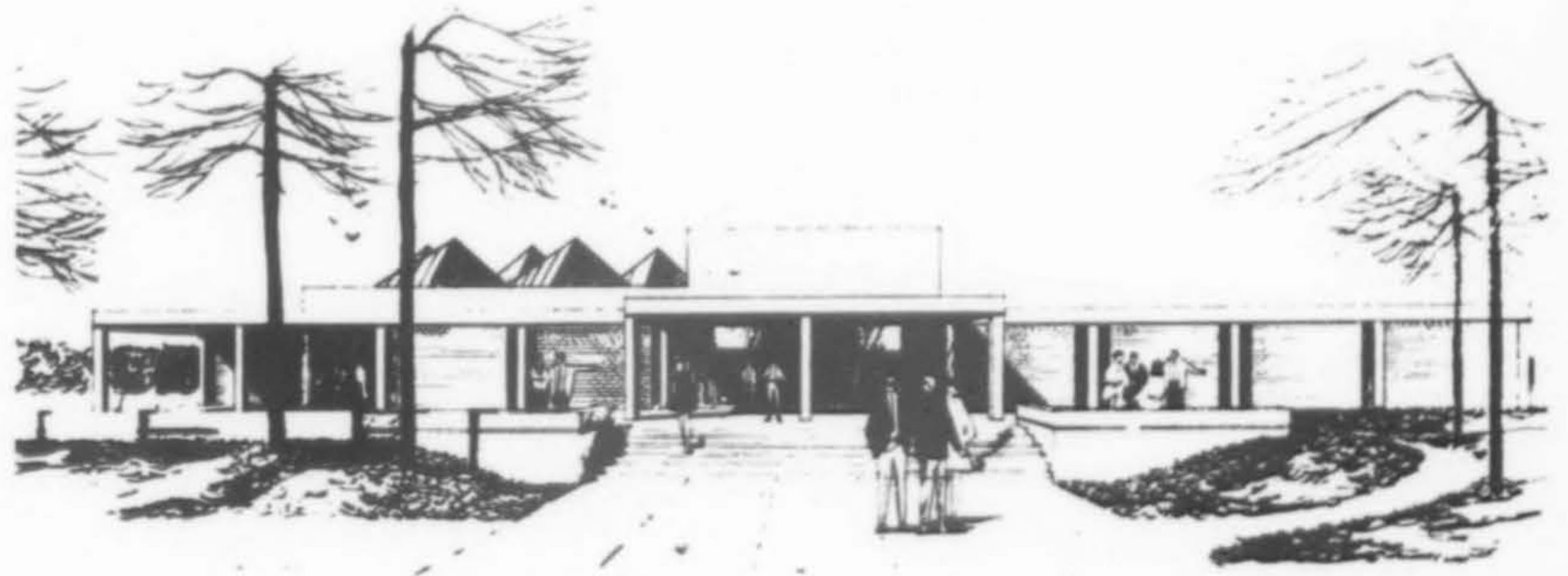
Cafeteria building, Sonoma State College, Rohnert Park, California, faces onto the main campus center. The building is surrounded on three sides by a terrace overlooking a man-made lake. The roof is composed of a series of light gathering monitors supported on a diagonal beam system allowing natural light illumination. Architects: Marquis & Stoller; Lawrence Halprin & Associates, landscape architects; Christiansen & Foster, contractors.
