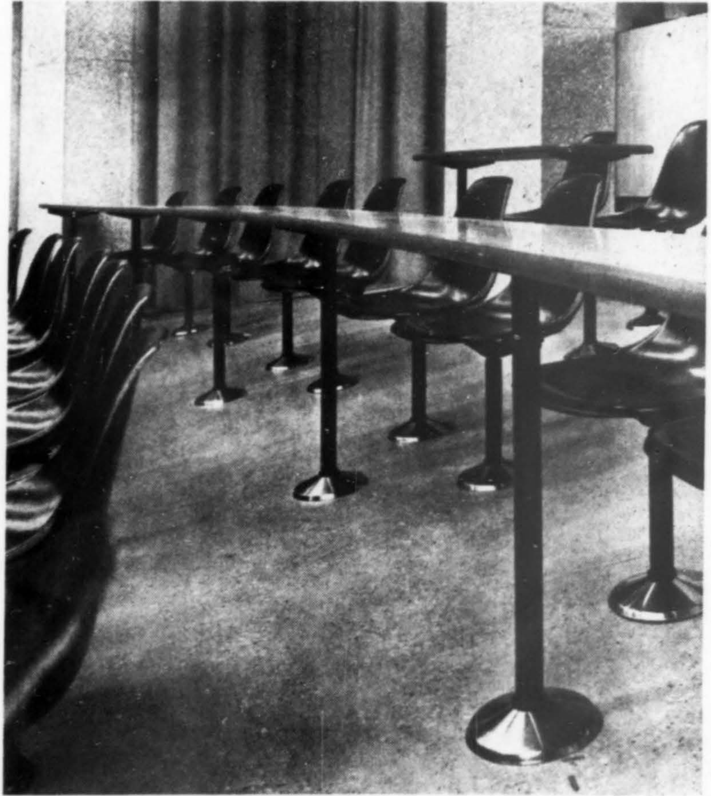
Science room has Herman Miller's fixed tables and pedestal-base chairs. Units are angled to fit inclined floor; the alignment of the radius of the top surface is accomplished by template.
