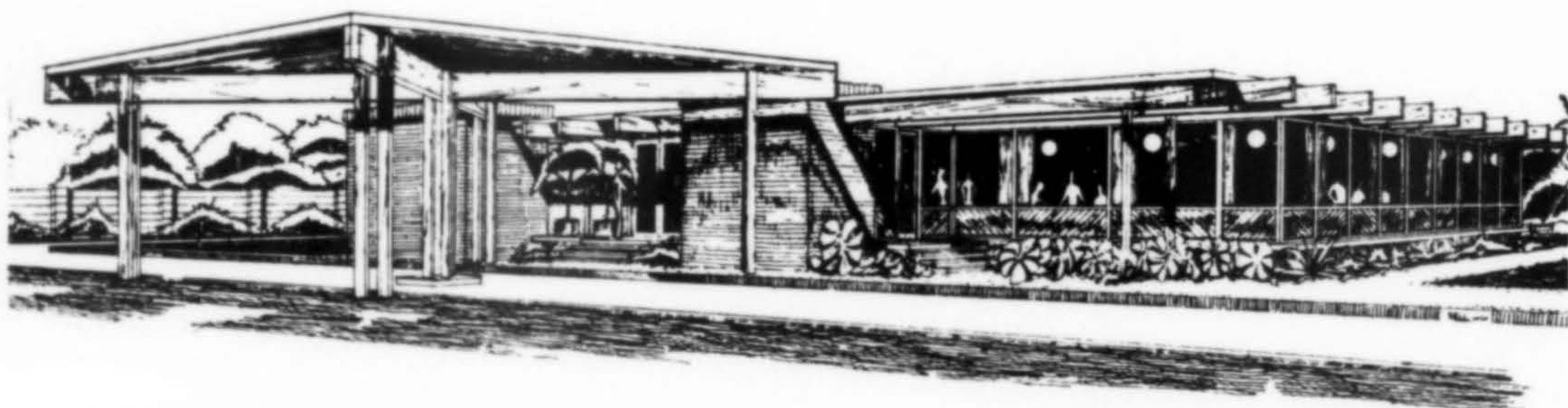
WALKERS THOMAS EAST Restaurant, Phoenix, Arizona, will be built in conjunction with 495 unit apartment and office complex adjacent. The 7,500 sq. ft. structure will seat 400 in coffee shop, dining room, lounge and private rooms. Construction will be slump block and stucco with glu-lam beams and wood decking. Architects: Donald B. Schwenn & Associates.
