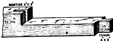
Splicing Timber.—Fig. 1.—Half of the Splice.
