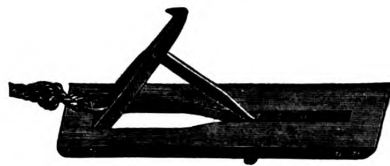
Fig. 16.—Scaffold Bracket Ready for Plank.
