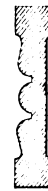
Section of Inside Casing of Doors and Windows.—Scale, 3 Inches to the Foot.
