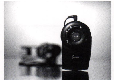
The Audible MobilePlayer, designed and developed by IDEO, downloads recordings from the World Wide Web and then uses RF (radio frequency) technology to play back the recordings through regular car radios. (photograph by Steven Moeder)
