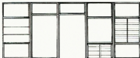
PANEL DISPLAY CASE PANEL PANEL WINDOW DOOR WINDOW JALOUSIE PANEL WINDOW PANEL LOUVERS PANEL
