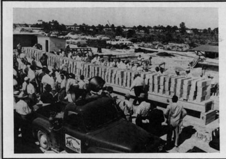
Load Test on 60-foot-long Channel Roof Slab produced in the "Double Tee" pre-tensioning bed at the Pompano Beach plant of R. H. Wright and Son. Conducted during 1955 Annual Convention of Prestressed Concrete Institute.
