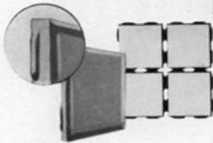
Stylon "Sure-Space" lugs project on all four sides of Stylon  $4\frac{1}{4}'' \times 4\frac{1}{4}''$  wall tile and crystal-glazed floor tile. Because these projections make true alignment and proper setting automatic, they're an assurance to the architect that his design will be executed exactly as planned.
