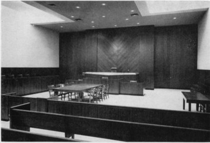
A typical Circuit Court Room. This is paneled in quartered and plain sliced walnut. All major rooms in the building are paneled — all with American woods.
