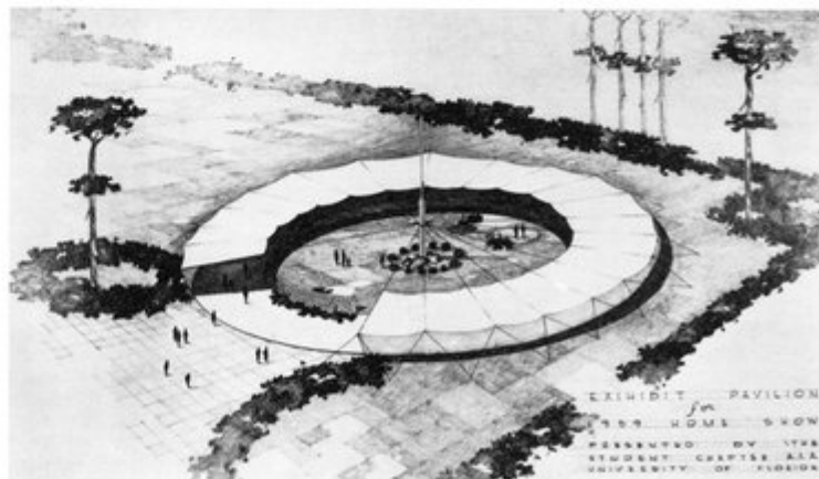
The Student Exposition Shelter will be a unique circular structure 160 ft. in diameter. Tensioned wires radiating from a central pylon will support a plastic membrane. Design and construction are in charge of Nelson Weller and Jay Dustard.
