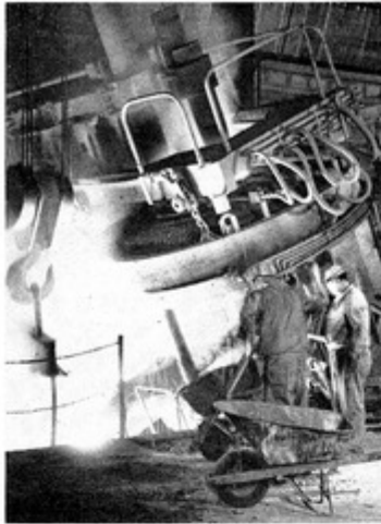
• 15 tons of molten steel pour from the huge electric furnace at Florida Electric Steel Mill in Tampa.
