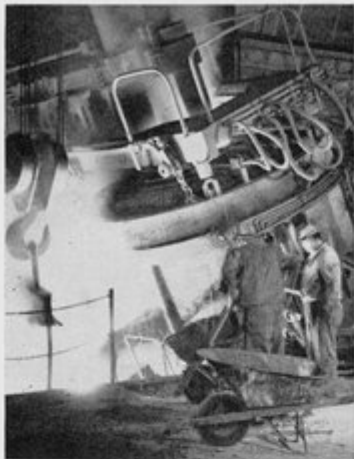
• 15 tons of molten steel pour from the huge electric furnace at Florida Electric Steel Mill in Tampa.
