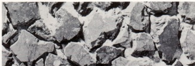
RUVIDO MISTO LUCIDO. As above, with aggregate surface ground and highly polished.
