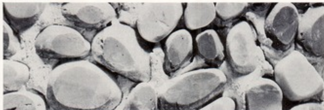
GLOBO MISTO LUCIDO. As above, with aggregate surface ground and highly polished.
