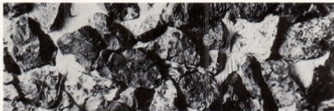
RUVIDO MISTO. Rough aggregate in mixed sizes. Shown one-half of actual size.
