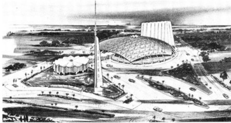
In Florida, as elsewhere, Fuller's principles of geodesic design are being recognized as a unique solution to a whole series of spanning problems. As one example, this sketch for a Metropolitan Amusement Center for Fort Lauderdale embodies a geodesic dome 400 feet in diameter which is now being engineered in aluminum by the Kaiser organization to house 15,000 people. Charles F. McKirahan, AIA, and Associates are the architects.
