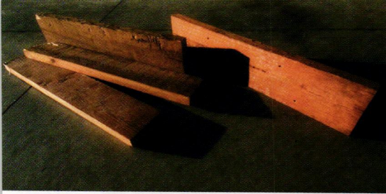
Wooden boards salvaged from the original building. These boards were ripped down to various thicknesses and stacked to create the feature wall. PHOTO BY JAMES CORNETET.
