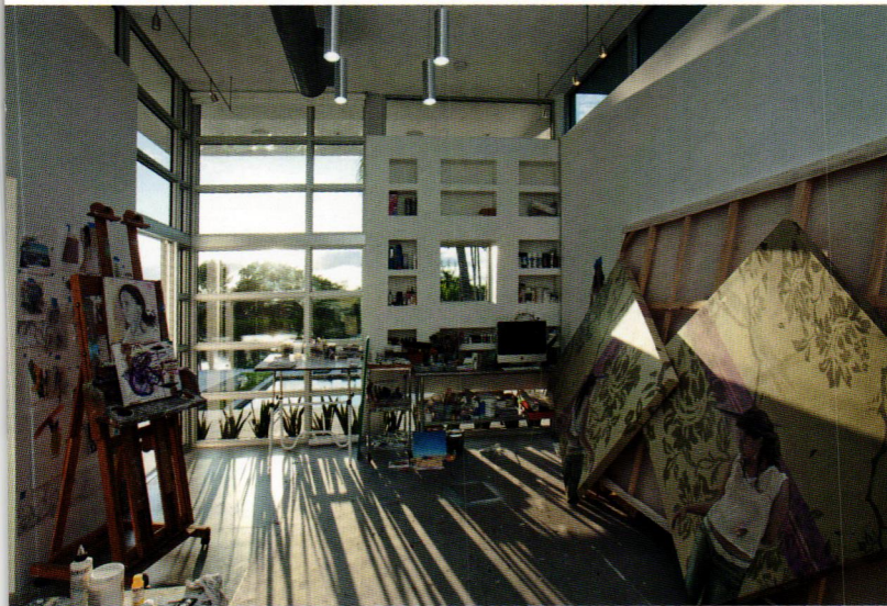
Studio windows rise the full height of the walls to admit the maximum amount of natural light.
