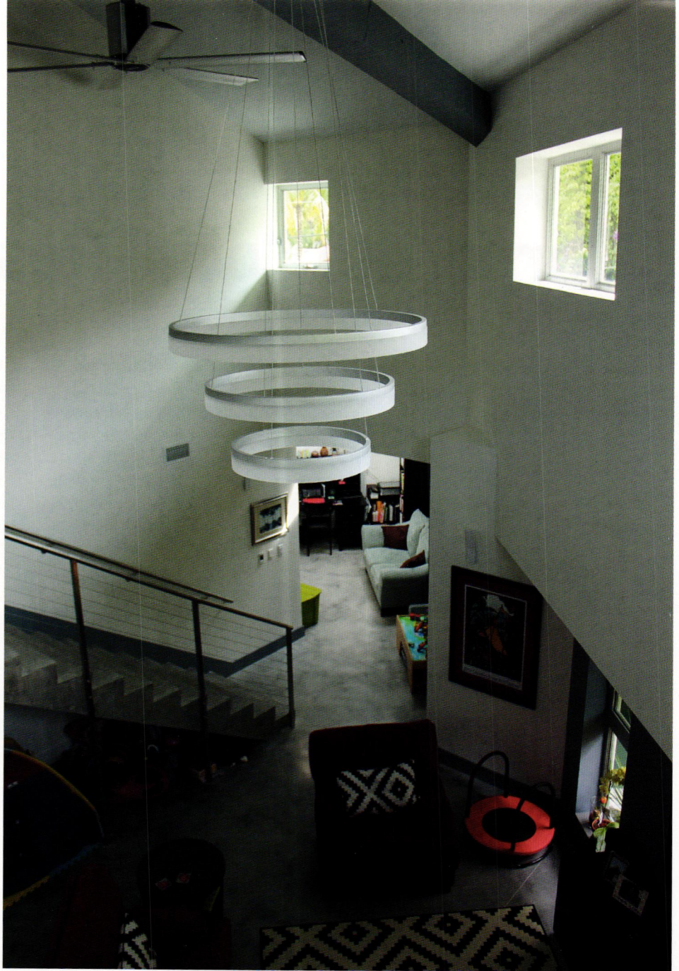
The Florida vernacular-style house was designed to create a natural air-conditioning effect through the use of operable windows and vaulted ceilings with high-volume, low speed fans.
