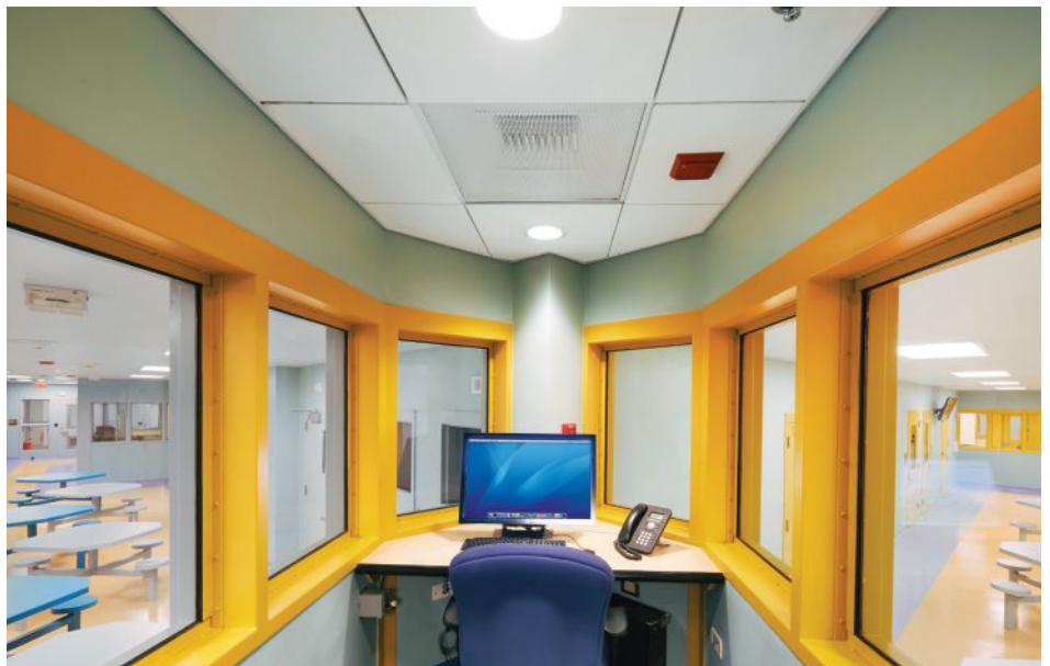
The nursing and security stations are located at the corners of V-shaped corridors so that both medical and security personnel can observe all patients at all times.
