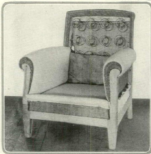
The second stage includes the back springs and the layers of burlap stuffed with hair and sewn in place
