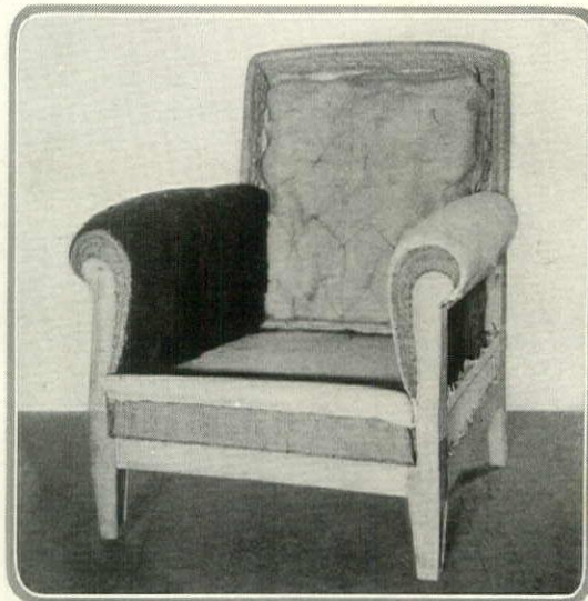
The third process finds the arms covered with a layer of down sewn in a stitched edge and the back completed
