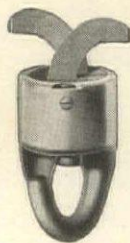
Front view of Elexit receptacle. This universal receptacle with circular or rectangular plate can be attached to virtually all types of outlet boxes in either walls or ceilings—ready to receive instantly either of the Elexit fixture supporting plugs shown, or the standard attachment plugs now found on electrical appliances.
