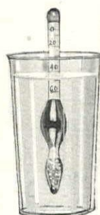
An hydrometer to test the consistency of liquids
