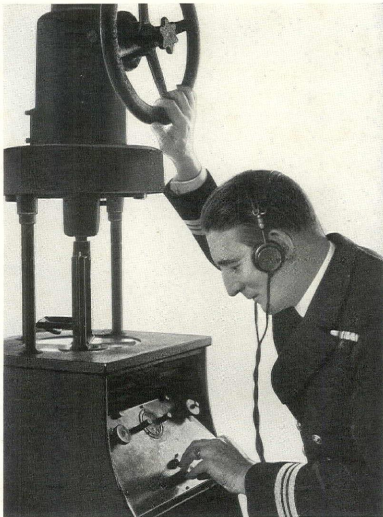
The radio direction finder. Simple in principle, this recently perfected device determines by relative intensity the direction in which wireless waves are traveling. Two or three land stations are tuned in and the directions of their signals noted. Then, on a chart, lines are traced out to sea in the indicated directions from the known stations. The point where these lines converge is the ship's position.
