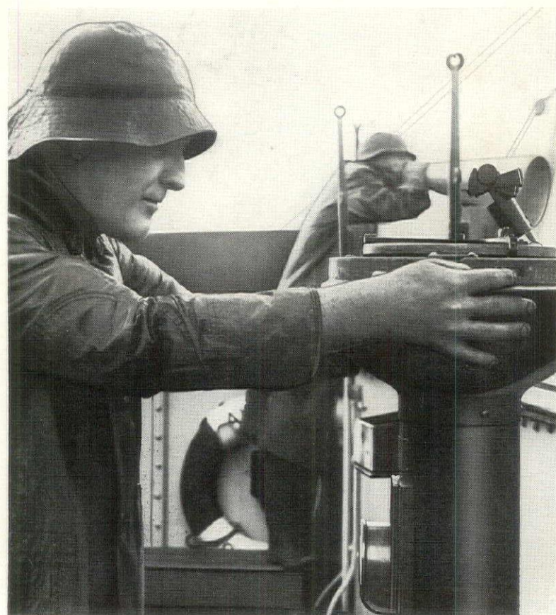
The Aquitania meets a squall. The Captain has just altered the course 10 degrees to starboard and the Junior Officer of the watch is checking the new course by the "repeater gyro" . . . a compass controlled by the master gyroscope below decks.
