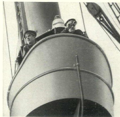
The Crow's Nest. In Cunard ships, at all times, two specially trained lookouts are stationed here. They are equipped with high-powered binoculars and a loudspeaker telephone to the bridge.
