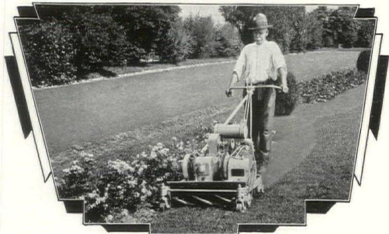
Above: Goldwell "Train-Thirty" motor lawn mower and roller. Mows and rolls simultaneously 6 to 8 acres a day.
