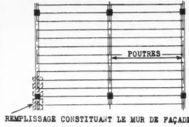
BATIMENT A OSSATURE
