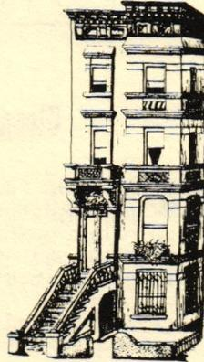
**S**ANDSTONE (also called "brownstone") was a popular building material in the 19th century. Quarried in the Connecticut River Valley and in New Jersey, sandstone was easy to cut and carve when fresh from the quarry. Upon exposure to the air, the surface crystallized making it much harder.
