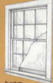
To evaluate the window's weather seal, determine if condensation is appearing on the sash glass or on the storm.
