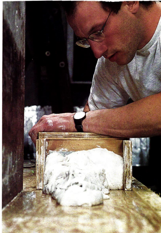
Left: As Frank lays the first batch of plaster, it pours out of the bucket at roughly the consistency of cake frosting. Above: Part of the skill of running the mould is keeping the two vertical slippers in constant contact with the bench and tight against the lattice (right in photo) while it pushes through the slippery plaster.
