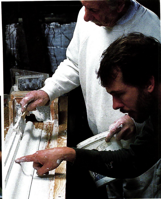
Below: In under an hour, a bucket of wet plaster has been transformed into 8' of moulding with skin-smooth curves and corners as sharp as glass. Bottom: A gentle nudge releases the finished moulding, and readies the bench for the next run.
