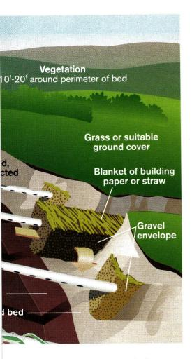
pipes, and laterals. Grass is the best vegetative cover for the disposal field. Also, don't drive vehicles or heavy equipment over the disposal field.
