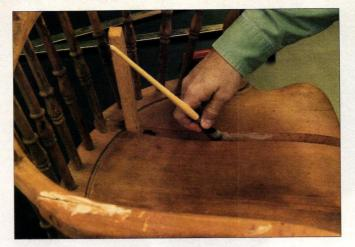
Though hide glue is the adhesive of choice for fine furniture, yellow, PVA-based "carpenter's" gluedesigned for most woodworking projects-is not as runny on vertical surfaces. This characteristic is enhanced for moulding and trim alue products.
