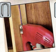
Install wire & cable with 4 sizes of Round Crown Staples
