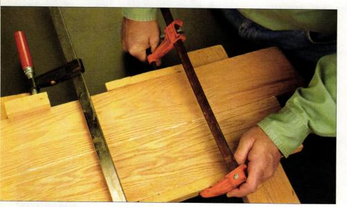
Good clamping ensures that the adhesive is completely distributed throughout the joint, and that the parts will not migrate out of position before the adhesive sets.
