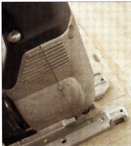
Sawing from the hole along the scribed line completed the cut. The scheme of 24" and 12" cuts was planned to take advantage of existing joints in the staves.
