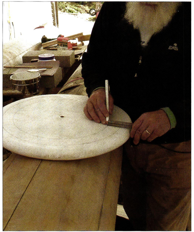
The circular rabbet or channel that was added to each plinth holds the staves together.
