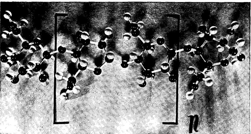
*Figure 1—single-molecule chain in cellulose fiber is made up of hexagonal units formed by five carbon atoms and one oxygen atom (above). Each unit contains three hydroxyl groups of one oxygen atom and one hydrogen atom.*
