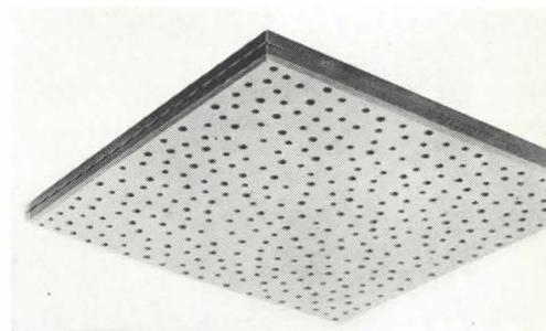
**Acoustic Tile:** "Full Random"/ nondirectional perforation design in "Cushiontone" fiber tile/ narrow bevel edge/ white-painted surface reflects 78% of light that strikes it/ washable/ available with flame-resistant-paint finish/ 12" squares in 1/2" and 3/4" thickness/ **Armstrong Cork Company, Lancaster, Pa.**
