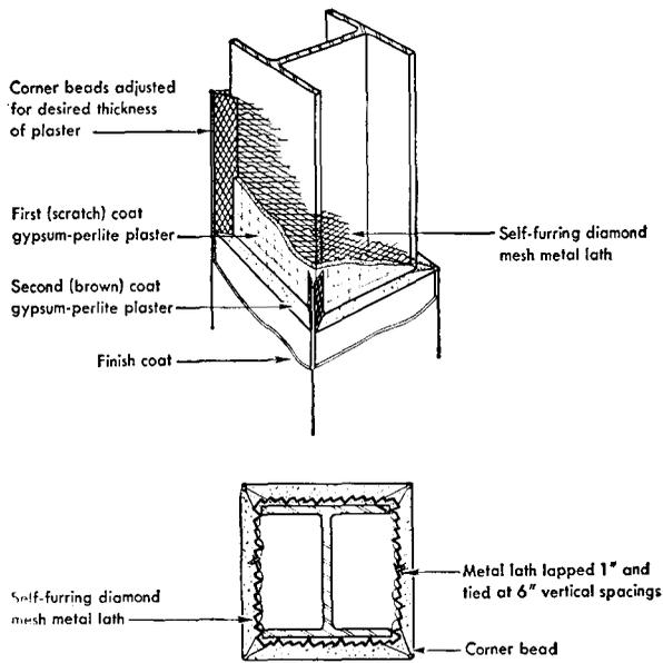
A new method of fireproofing steel columns, developed and tested at the Underwriters' Laboratories, employs light-weight-aggregate plaster and self-furring metal lath bent to fit columns. Indentations in the lath hold it  $\frac{1}{4}$ " from the steel surface, providing space for the plaster to key. No channel furring is required. Metal Lath Manufacturers Assn., Engineers Bldg., Cleveland 14, Ohio.
