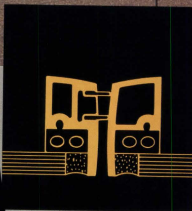
Adjustable astragal at meeting stiles for thermal integrity.
