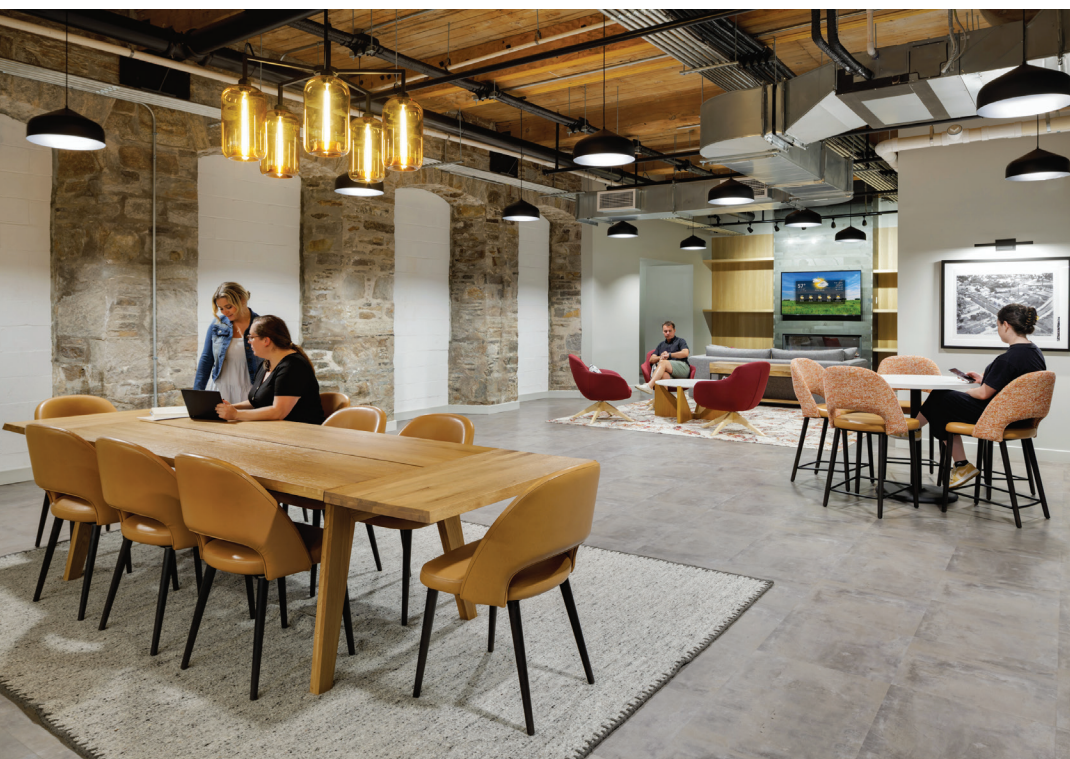
Amenity spaces were strategically placed at subterranean locations, so the exterior stone wall could be left exposed with limited energy loss.
