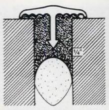
The masonry-joint protective system from WEATHERCAP, INC., is a soft lead strip embedded in caulk to form a cap or seal for any masonry joint. The type A flat cap is shown, for use in joints on the same plane. Write in No. 504
