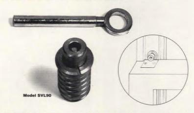
Our Model SVL90 secure ventilation lock is designed to limit opening of a doublehung wood window to an amount adequate for ventilation. The lock has a solid, machined brass housing and bolt. Included with each lock is a steel operating key and a brass strike plate for mounting on the lower sash check rail.
