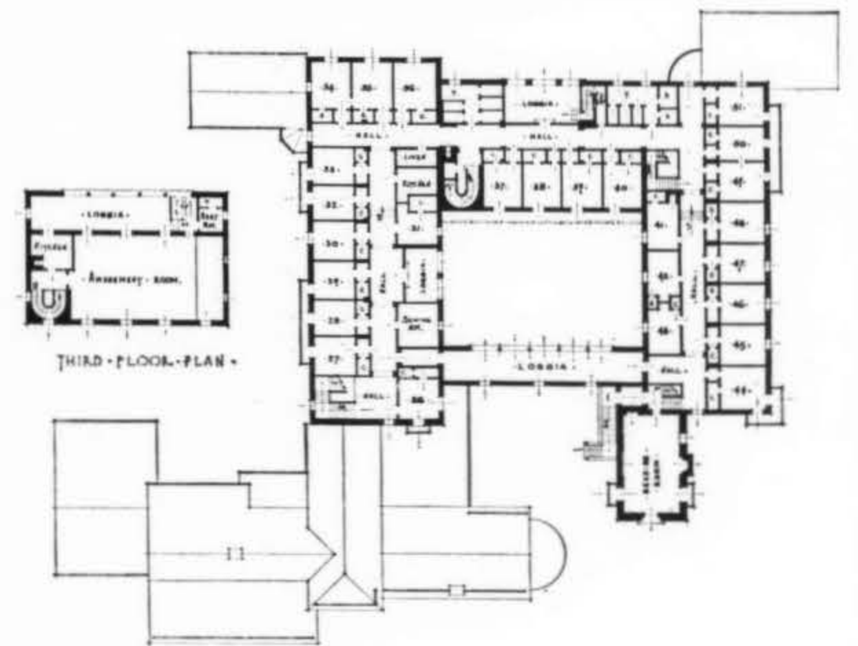
Floor plans of Toll Hall show the disposition of the rooms around courts and terraces, with loggias and balconies, with varying heights of the different wings, all combined into a grouped mass of charm and character. Gordon B. Kaufmann, Architect. Wurster Construction Company, General Contractors.
