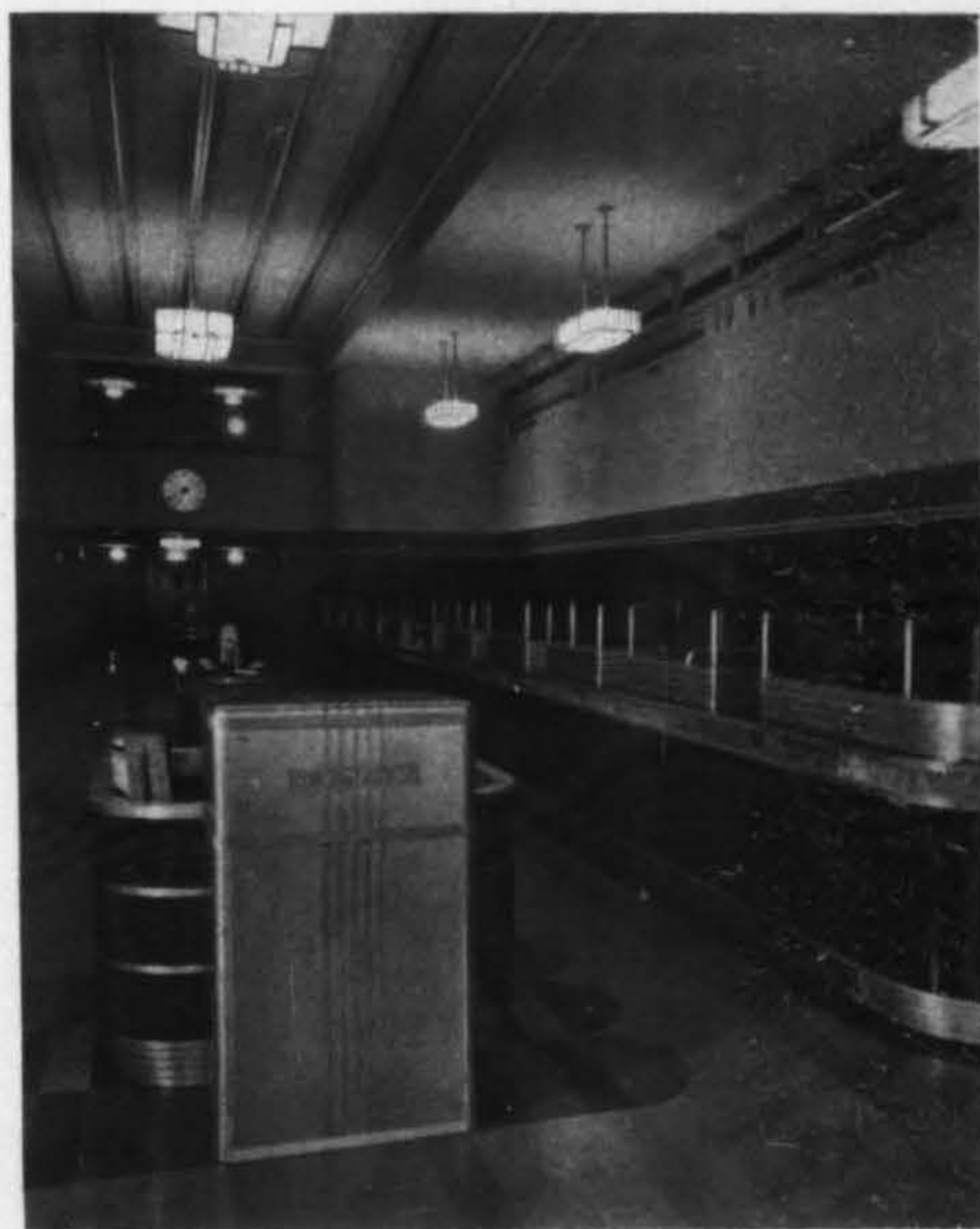
The main banking room is modern and especially pleasing. The walls are acoustic plaster tinted and decorated in water color. The floor is covered with sheet rubber in varying shades. The telephone switchboard at the information desk is housed in an ornamental aluminum cover. By emphasizing the longitudinal lines a feeling of greater depth is secured.
