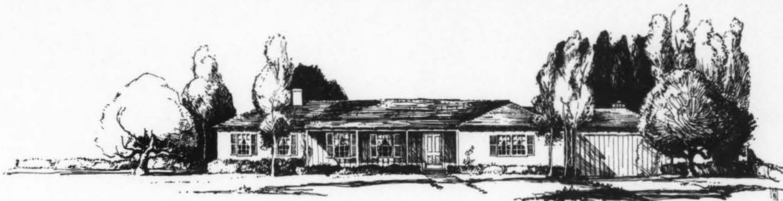
For a corner lot architects Erle Webster and Adrian Wilson have designed this six room house to cost $5,700. Of substantial wood frame, vertical board siding and stucco with shake roof, it will contain 1900 square feet.
