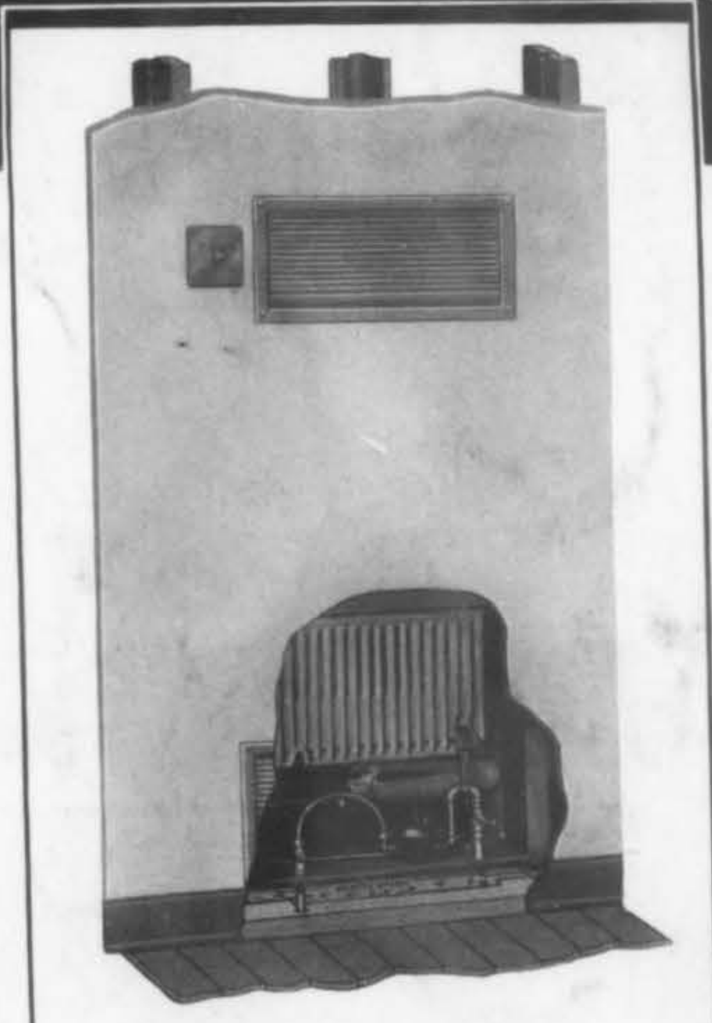
Front view showing upper grille and remote control, burner, cast iron fire box, safety valve, pilot and pressure reducing valve. Unit furnished with metal lath, front and back, for plaster, with lap-over to be nailed to studding. Overall size: 52½ inches high, 28½ inches wide, 9¼ inches deep.
