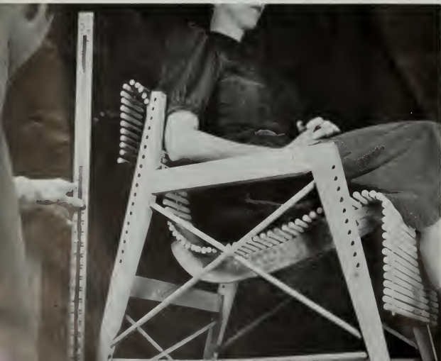
Determining the character of support needed by the body—the first step in designing a chair
