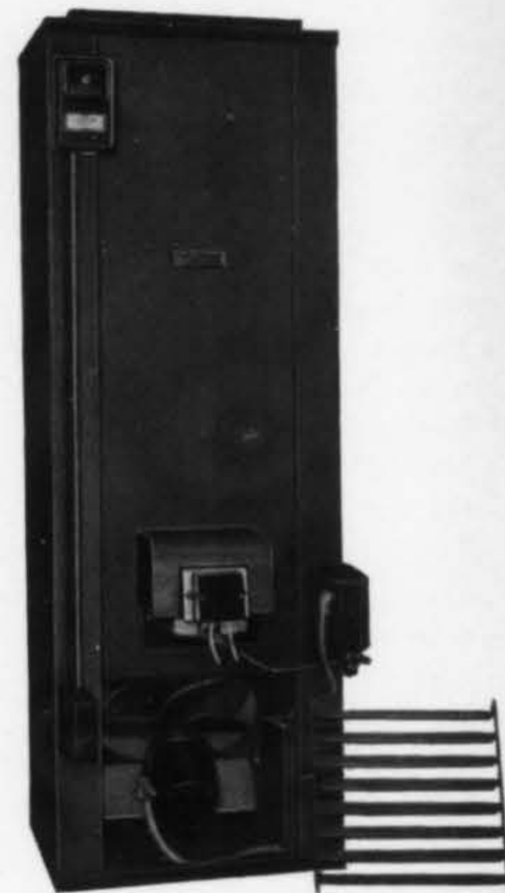
Oil-burning DU Furnace Burner unit with Electric Oil Control Valve, Electric Ignition and Automatic Fan and Limit Switch. The front grille is removed to show the Fan. Operation is entirely automatic, thermostatically controlled.
