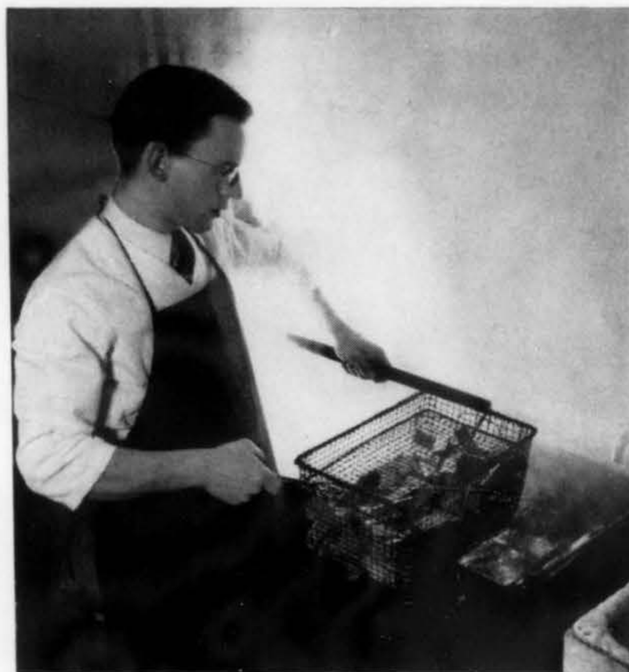
Boiling for betterment. Tiny samples of Douglas fir plywood, cut from thousands of random panels, each month are boiled and re-boiled as one test of the bond between plies in the exterior (waterproof) type panels. The samples are boiled for four hours, dried, then boiled again. While wet, samples are destroyed in a shear-testing machine; the wood itself fails while the glue-line or bond remains firm.
