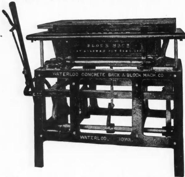
**ONE** movement of the lever operates the **ENTIRE** machine, consuming the least time for operation of any machine. Two men will make 250 blocks per day.
