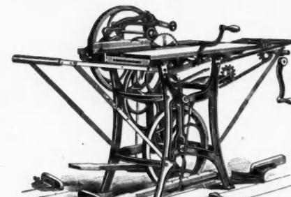
"Union" Combination Self-Feed-Rip and Cross-Cut Saw
