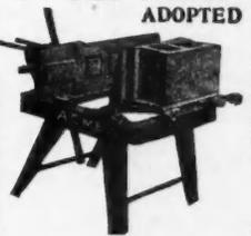
Notice the advantages offered in this machine, the practical points embodied, the great value it is. Makes blocks face down and in various sizes from 8x8x16 to 8x12x24. All on the same frame, with the substitution of plates. Either wood or iron pallets may be used, and blocks can be made with either a dry, medium, or wet mixture.
