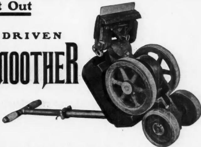
Meets every demand of practical men for a machine that will scrape and sandpaper a floor and do it right. It has all of the ready adjustability of a hand-scrapers—the necessary weight to keep it from jumping, and the motive power to enable the operator to do ten times the amount of work that can be done by hand.
