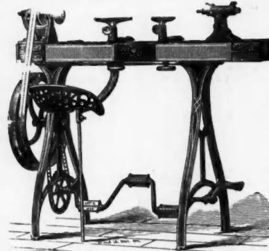
Our No. 3 Wood Turning Lathe can be speeded from 1,000 to 2,000 revolutions a minute with perfect ease. Stopped or reversed at will of operator.
