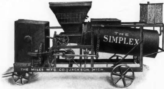
the fact that batch mixers are being made as near continuous as it is possible to make them. Often objections have been raised regarding continuous mixers, due to the unreliability of many, both as to feed and mix.
