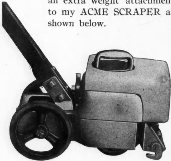
This extra weight adds 40 pounds pressure over the cutting edge of blade and will force the knife into the hardest wood surface. As this additional weight is only required while scraping old floors or some special grades of new hard wood floors, it is so constructed that it can be attached or removed in a few seconds time.
