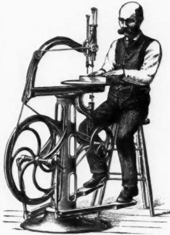
Suitable for carpenters, pattern and cabinet-makers and all wood-workers requiring accurate work, also for sawing soft metals. Will cut up to 3 inches thick, swings 24 inches, has powerful tread motion, cuts rapidly and is easy to operate. Has adjustable tension spring on upper spindle, dust blower, drill attachment, iron tilting-table, etc. Will furnish tight and loose pulleys for power in place of treadles when desired.
