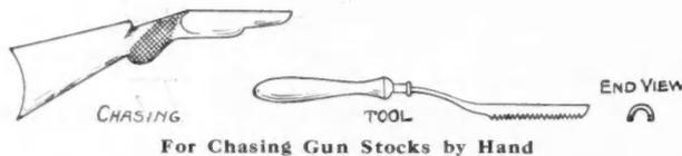
the same movement as you would with a file; and after one pair of creases have been cut, the last one can be used as a gauge to cut the others, which only gives one cut or crease at a time. Then cross cut the same way; the edges of the tool should be sharp and cut with teeth similar to a fine saw.
