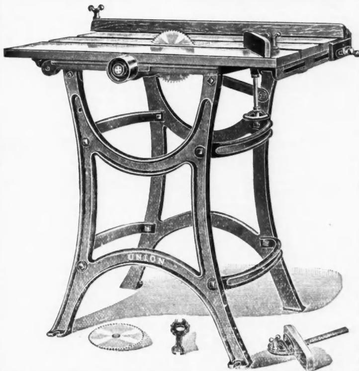
A well-built, light power machine, at a low cost, has a wide range for work, will rip stuff up to 3½ inches thick, also cut off, mitre, and with attachments, bore, edge-mould, groove, dado, etc.
