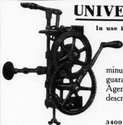
Will cut lock mortises, including setting in of face plate, in any desired size, in hard, soft or cross-grained wood of every description, in from 3 to 6 minutes. No boring or chiseling required. Every machine guaranteed. Makes a perfect job. Easily operated. Agents wanted where not represented. Testimonials and descriptive booklets furnished on application to
