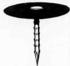
Roofing nails are for paper, not metal, hence a large head is required. The Simplex has a head surface four times that of a so-called large headed nail. Head surface is what holds down roofing. Insist that the roofing comes to you with Simplex Nails. They are time savers as well as having head surface. Made with 1 inch and 1 3/8 inch lengths of stem, and both plain and galvanized. Shipped in cans in prepared roofing—store stock in 100 lb. kegs. Sold by dealers and jobbers.
