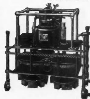
Rapid and Flexible Stone Floor Surfer for Concrete with Terazzo, Mosaic Tile, Cement, etc.
