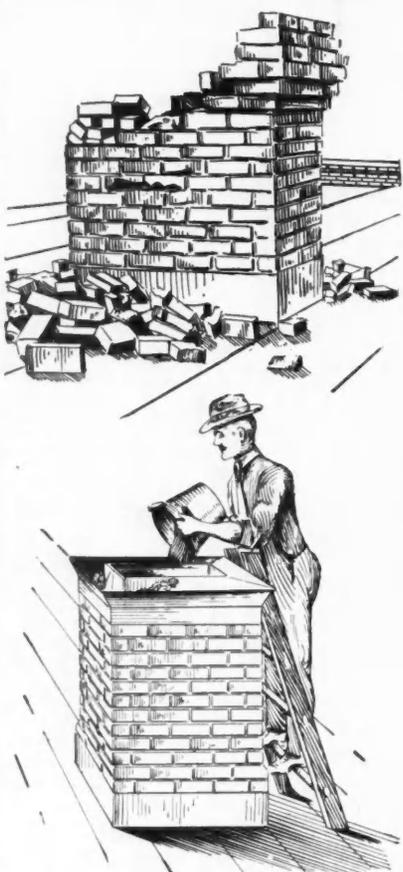
Simple device for prolonging the lives of chimneys. Made from cast iron.
