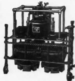
Rapid and Flexible Stone Floor Surfacer for Concrete with Terrazzo, Mosaic Tile, Cement, etc.
