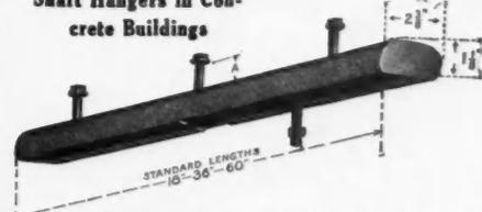
Trus-Con Pressed Steel Inserts are embedded in the concrete during construction, saving expensive drilling after completion of the work. The long slots allow a wide variation in position. Special washers prevent bolts from turning in the slots. Write for details and prices.
